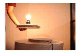
Fig.1: Wireless power transmission
