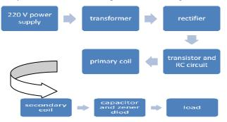
Fig.4:Block Diagram of Wireless Transmission
