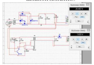
Fig.3: Circuit Simulation on Multisim Software
